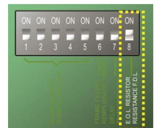
**Figure 18: End of line resistor switch in position "ON".**
