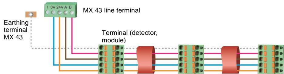
Figure 16: Principle of connecting modules to a MX 43 line.
