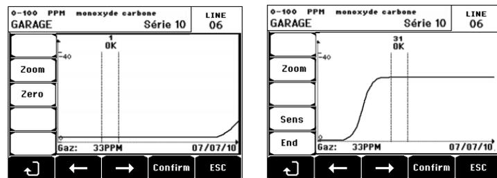
Figure 48: Adjustment of zero (left) and sensitivity (right).
