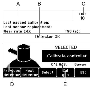
Figure 47: Example of the “Select detectors” screen.
