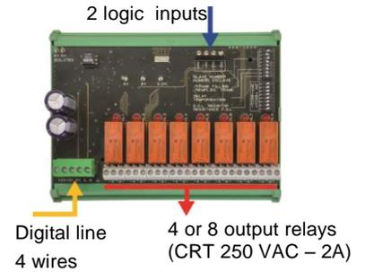
Figure 19: 8-relay module.
