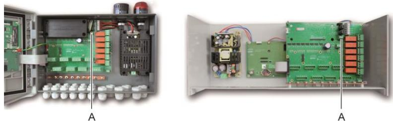
Figure 29: Connection of 24VDC external power supply (A).
