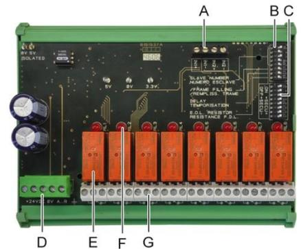
Figure 20: 8-relay module.
