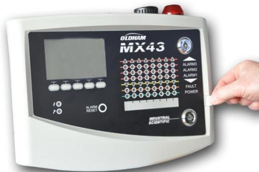
Figure 13: Pulling the tab.
