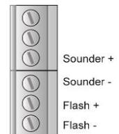
Figure 36: Flash and siren connector (A).
