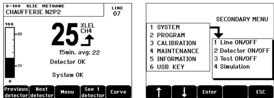
Figure 12: Example of a measurement display (screen) or parameter setting display (menu on the left).
