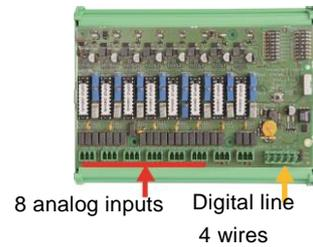
Figure 23: 8-analog inputs.
