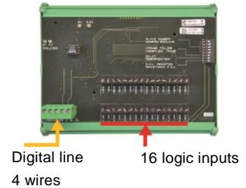
Figure 21: Module with 16 logic inputs.
